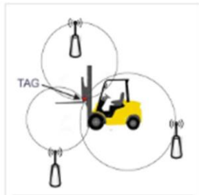
Real-time locating systems (RTLS)
